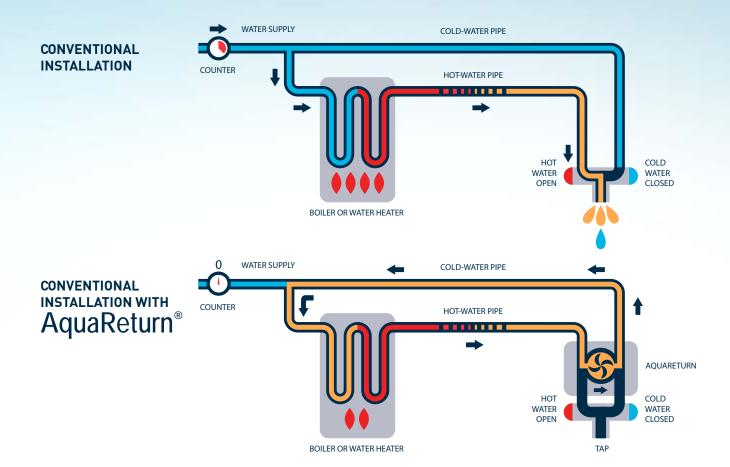
To activate AquaReturn, simply turn the hot water tap on and off at the sink where AquaReturn is installed. The appliance has a mechanism that stops water flowing from the tap until it has reached a temperature of 35°C (95°F) or 25°C (77°F) depending on the market. Once the water is hot enough, a beep will tell you that hot water is now available from any of the taps in the bathroom.
